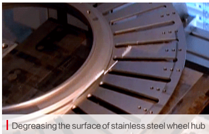
Degreasing the surface of stainless steel wheel hub
